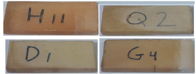
Fig.5 some samples after efflorescence test
