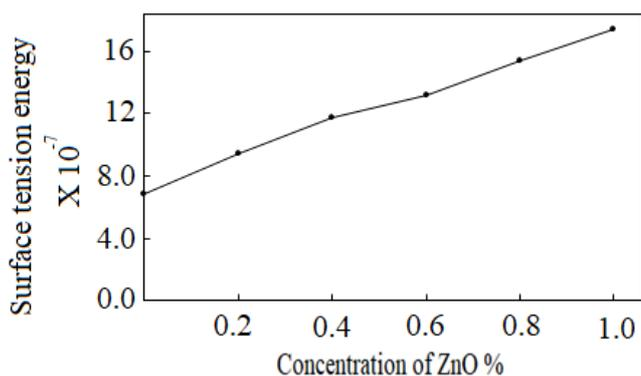
Figure.11. Surface tension energy vs. different concentration of ZnO nanoparticles for PVA/ ZnO nanoparticles solutions at 30°C.
