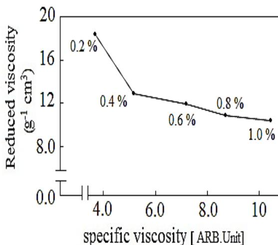
Figure. 7. Reduced viscosity vs specific viscosity nanoparticles for PVA/ ZnO nanoparticles solutions with different concentration of ZnO nanoparticles at 30°C
