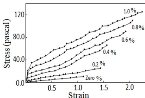
Fig2: The effect of concentration of ZnO nanoparticles on stress-strain curves for PVA/ ZnO nanoparticles thin films.
